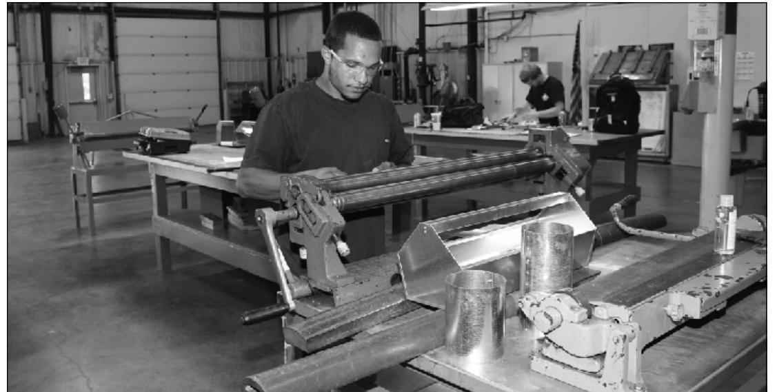
AT WORK ON AN OGEE OFFSET duct at the Local 7-Zone 1 Training Center in Coldwater is sheet metal apprentice Caleb Burnette.
