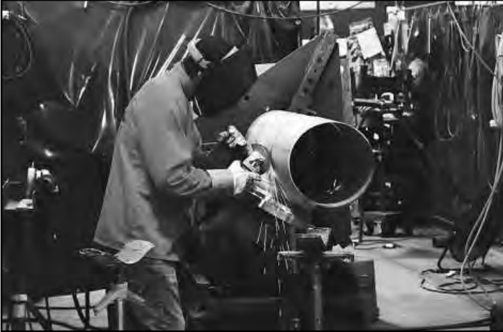
FABRICATING STAINLESS pipe for use at the Saline Wastewater Treatment Plant are (l-r) Ryan Goggins and Sean Newman. The Plumbers and Pipe Fitters Local 174 members are working at the Grand Rapids shop of Andy J. Egan. Photo credit: Andy J. Egan
