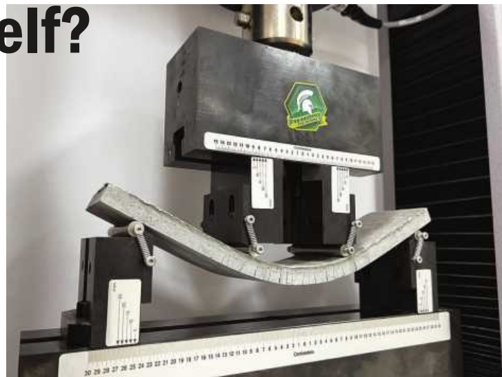
WELL, THIS LOOKS promising: concrete is tested at Michigan State University, giving engineers an idea of what mix offers the best bendable qualities.
